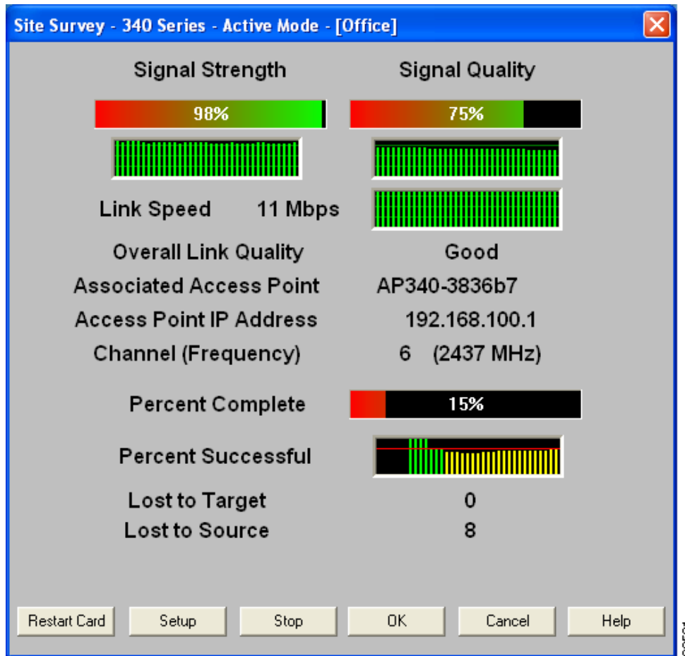
Figure F-4 Site Survey - Active Mode Screen (with Signal Strength as a Percentage)
