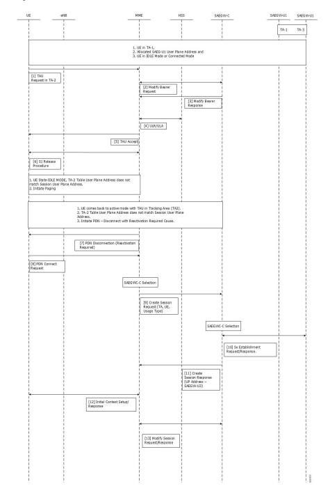
Figure 3: Attach in TA-1, TAU from TA-2, IDLE Mode and TAU in TA-3
