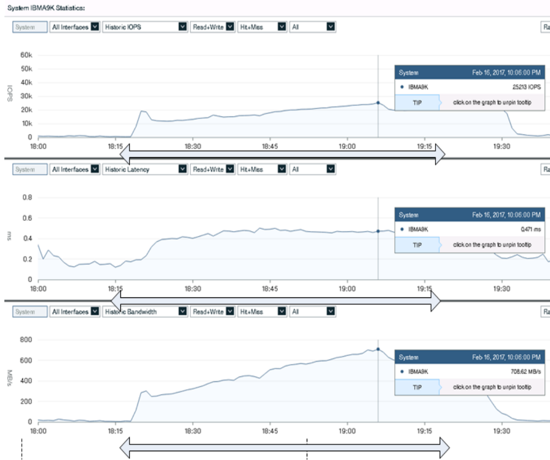
Figure 116 IBM FlashSystem A9000 Storage graphs for Latency , bandwidth and IOPS for 2100 Users RDSH Cluster Test
