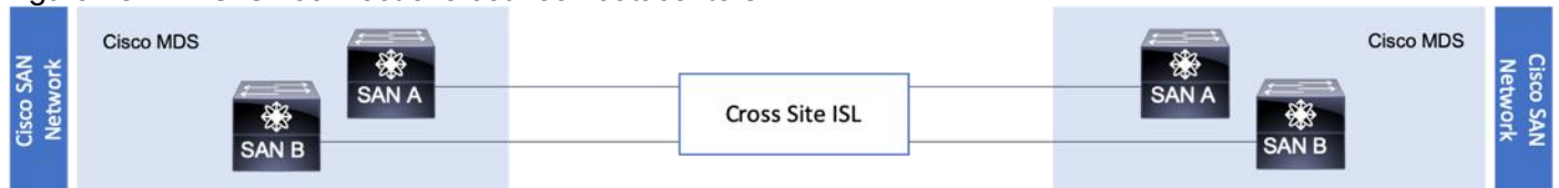
Figure 28 MDS ISL connections between datacenters
