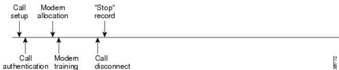
Figure 90: Modem Dial-In Call Setup Sequence With Call Disconnect Occurring Before User Authentication and With Resource Failure Stop Accounting Enabled
