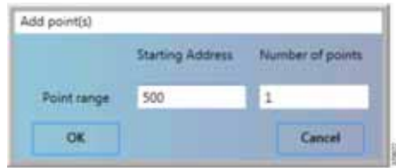
Figure 130 Eximprod IED Data Point Register Configuration
