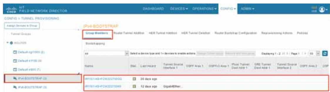
Figure 30 CHANGE Tunnel Group—Devices Moved under IPv4 Group
