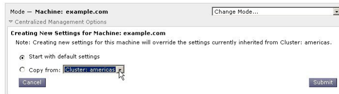
Figure 82: Centralized Management Feature in the GUI: Create New Settings
