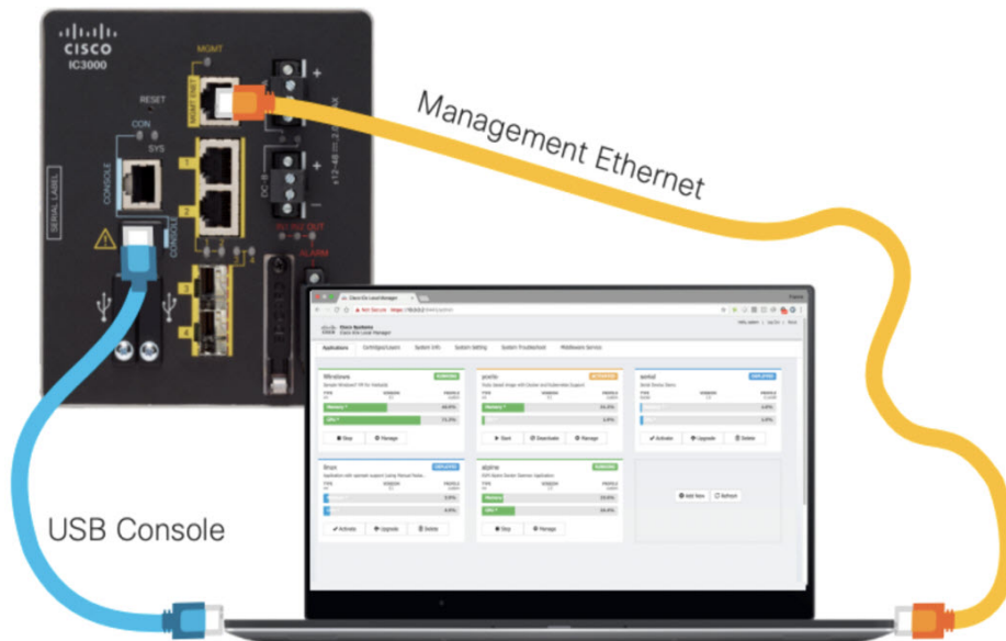
Figure 20: PC Connected to Management Interface
