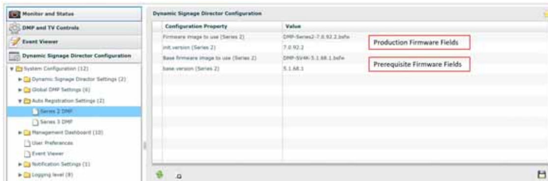
Figure 36 Firmware Image and Version Properties Required to Provision the SV-4K and DMP-2K
