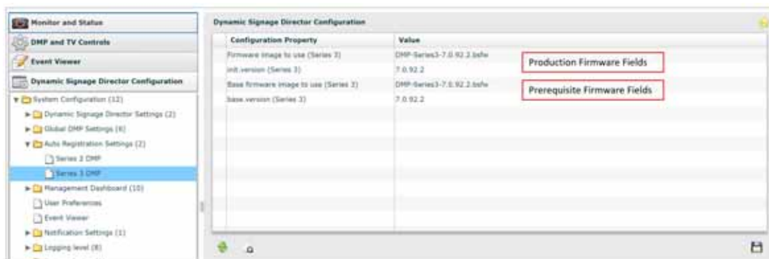
Figure 35 Firmware Image and Version Properties Required to Provision the CV-UHD and CV-HD
