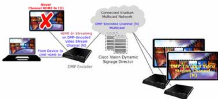
Figure 11 Unsupported DMP Encoder Configuration for HDMI-In Streaming
