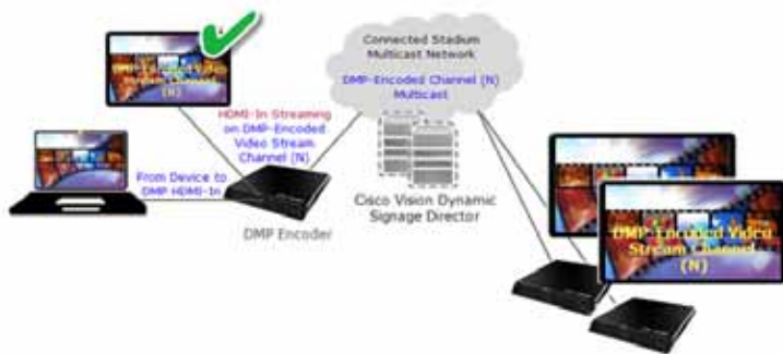
Figure 12 Supported DMP Encoder Configuration with TV Display for HDMI-In Streaming
