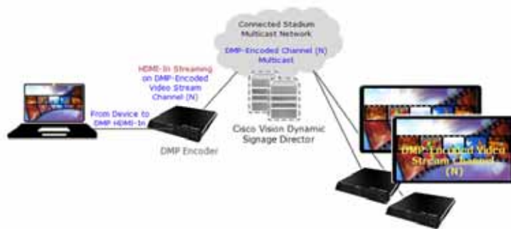
Figure 10 HDMI-In Streaming Example from Single DMP to Multiple DMPs
