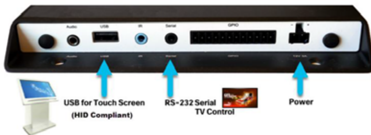
Figure 5 CV-UHD2 DMP Rear Panel Overview
