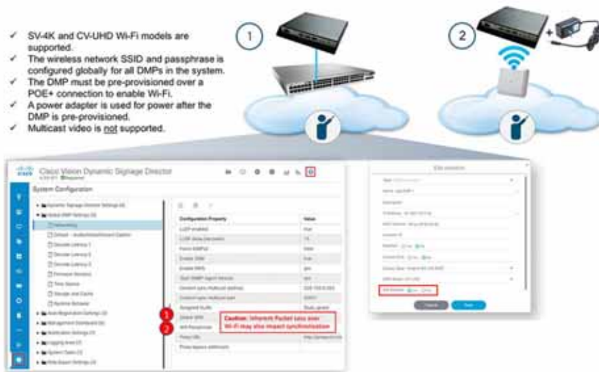
Figure 11 Connecting the DMP to the Wi-Fi Network Overview
