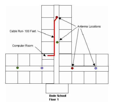
A coaxial cable carries radio frequency (RF) energy between the antennas and the radio equipment. An antenna cable introduces signal loss in the antenna system for both the transmitter and receiver. In order to reduce signal loss, minimize the cable length and use only low–loss (LL) or ultra low–loss (ULL) antenna cable in order to connect radio devices to antennas.
