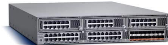
Figure 4. Cisco Nexus 5596T Switch Configured with Three 12-Port 10G BASE-T Expansion Modules
