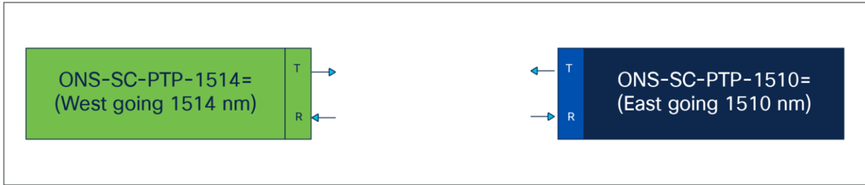
Figure 4. Depiction of the bidirectional functioning PTP DWDM SFP pluggable optics
