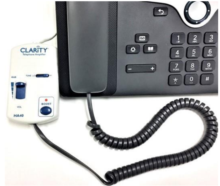
Clarity HA40 Inline Amplifier connected with Cisco IP Phone
