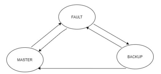
After the Keepalived pod is up and running, one of the RCM VM instances comes up as Primary and the other as Backup. When Keepalived health monitoring fails on Primary, it transitions to Fault state first and then to Backup state. At the same time, Backup transitions to Primary role. Whenever the state transitions to Fault state, the VM is rebooted. This action is done by keepalived\_notify script.
