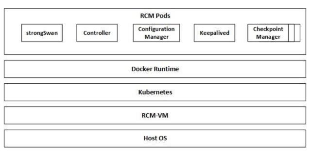
When RCM is deployed on bare metal, the RCM VM layer does not exist, and packet flow involves host kernel.
