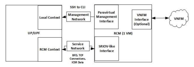
The RCM node is built on Subscriber Management Infrastructure (SMI). SMI provides the Kubernetes (K8s) infrastructure, which is used to bring all the required pods to support the redundancy for UPs.
