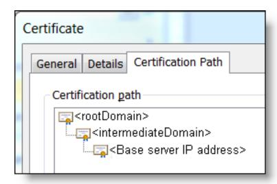
If the certification path is not correct, download the root and intermediate certificates again from the correct AD CS domains.
