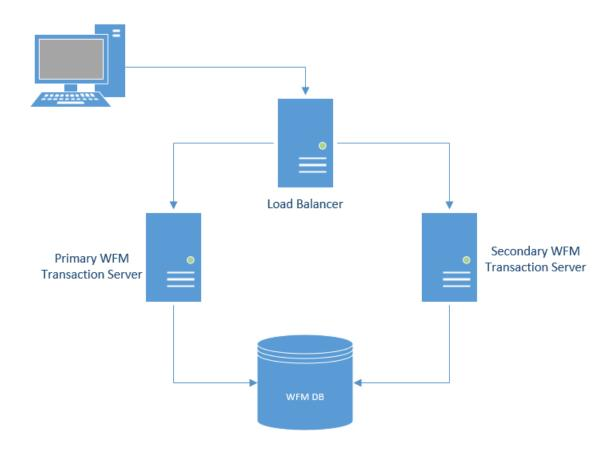
In this type of configuration, the load balancer provides a virtual IP address that the client browsers connect to. The load balancer forwards browser requests to the primary Transaction server if it is up, or to the secondary Transaction server if it is not.
