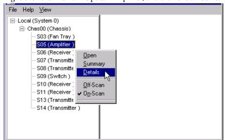
**Result:** The Module Details window appears. The alarms are shown under **Parameters** and **Alarms.**
