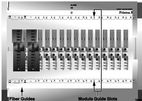
2. Align the ridges on the top and bottom of the module with the module guide slots located on the chassis. Module ejectors must be fully extended when inserting the module.
