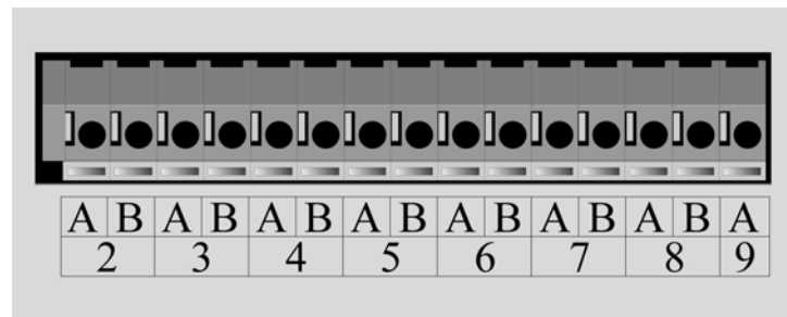
Close-up of Front Panel Terminal Strips
