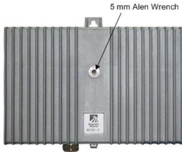
**Bolt Tightening position of the node type 90100**
