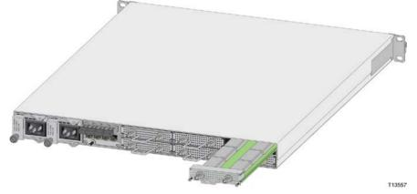
**2** Push the card in carefully making sure the QAM Card aligns with the system controller connector.
