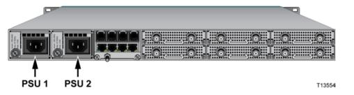
The following illustration shows the PSU installed.
