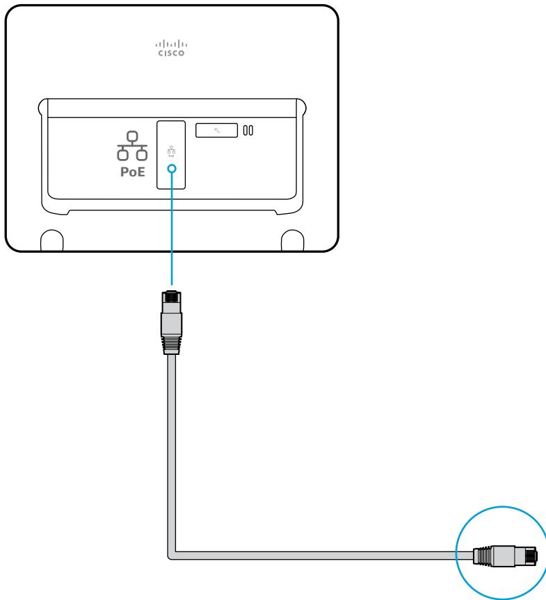
Connect to a PoE enabled network port on the video system (*direct pairing*) or LAN (*remote pairing*).
