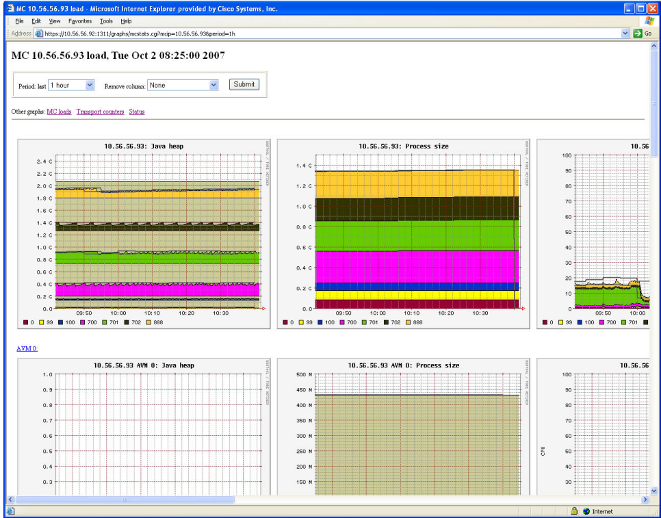
Figure 4-13 MC Loads Page—Drill-down to Specific Server
