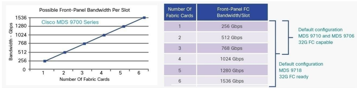
Figure 10. Bandwidth per Slot for Cisco MDS 9700 Series and Number of Crossbar Fabric Modules
